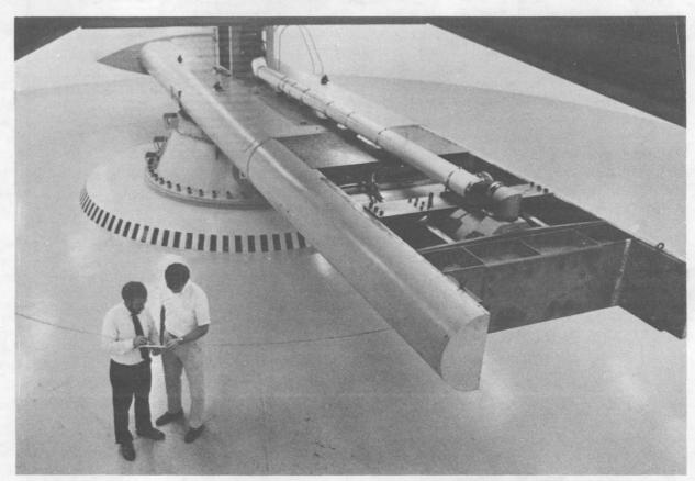
DAVE SCHAFER (7531, left) and Jon Rogers (7544) discuss details of the vibrafuge's performance. The shaker that provides the vibration is partly visible as a cylinder near the end of the centrifuge arm. The white pipe along the top of the arm carries cooling air to the shaker.
